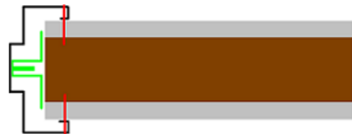
1 - Standard K.D. drywall frame assembly
