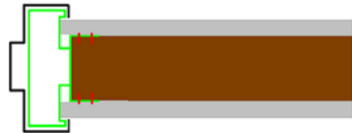
2 - Welded drywall frame assembly
